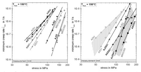
**Figure 5.** Minimum creep rates at a testing temperature of 150 °C versus stress for Mg- alloys processed by magnesium injection molding (left) and for comparison creep rates of AZ91 with Ca- / Sr-addition
