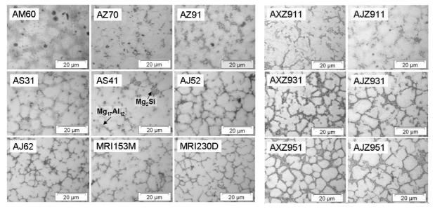
Figure 2. Microstructure of conventional alloys processed by magnesium injection molding.
