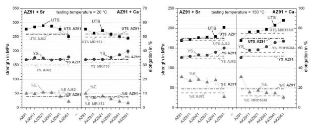
**Figure 4.** Mechanical properties at room temperature and 150 °C of AZ91 with Ca- and Sr-additions compared to conventional AZ91 and alkaline earth containing alloys AJ62 and MRI153M processed by injection molding.
