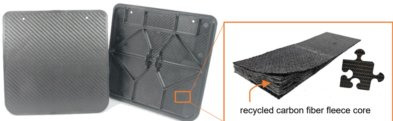
Fig. 1: JEC trade fair 2024 aviation demonstrator with recycled carbon fibre fleece core
