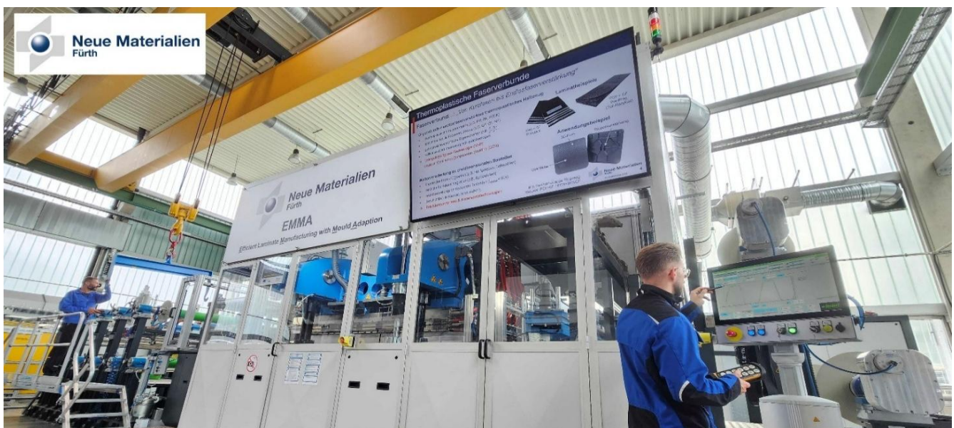
Image 2: 50-inch interval hot press with adaptive pressure optimization and fully automated release agent station at Neue Materialien Fürth's technical center
