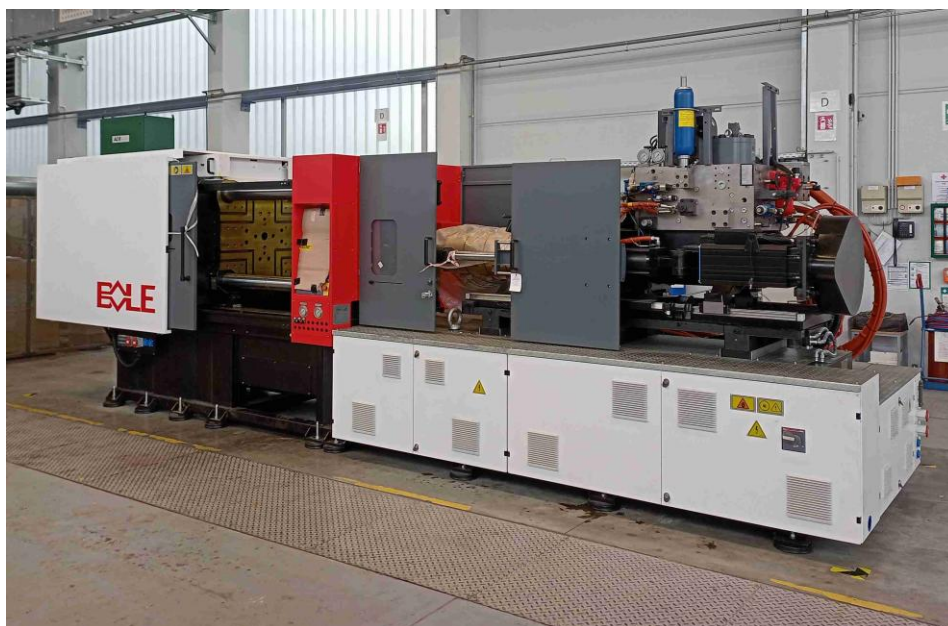
Figure 1: Installation of the Bole MTX300 Thixomolding machine at Neue Materialien Fürth GmbH is in progress.
