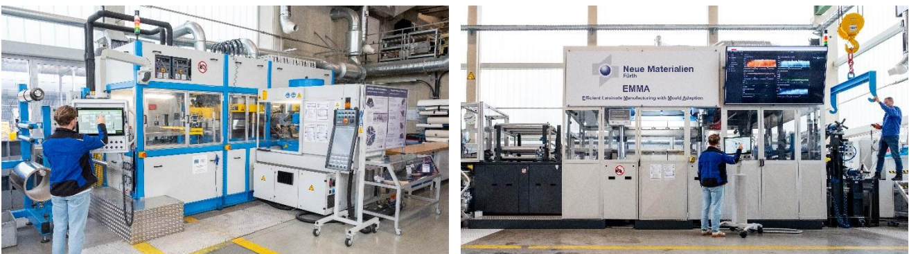
Figure 1: 25-inch CCM system with direct melt plasticization (left) and 50-inch CCM system with local pressure adaptation system (right) for the development and production of thermoplastic laminates
